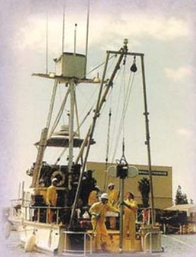
Vibrocore sampling for hazardous materials
